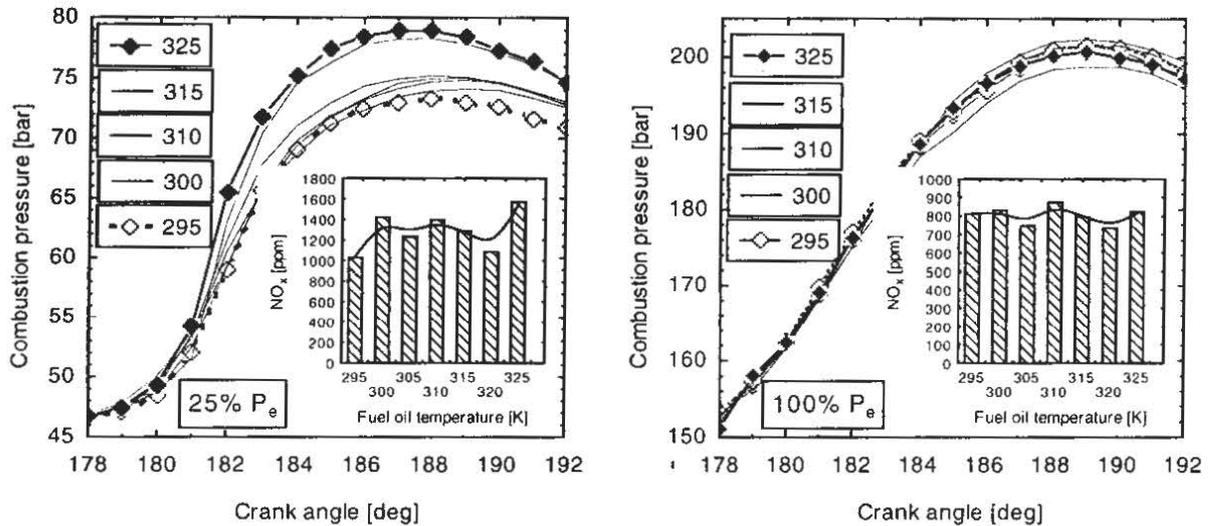
Figure 4. Calculated combustion pressure and  $\text{NO}_x$  emission profile of 8L32/40 engine fed by fuel oil with progressive rise of temperature (K) and for two loads 25% and 100%
