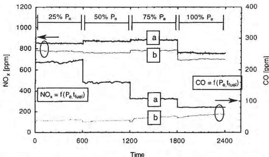
Figure 3.- Measured exhaust gas emission components profile of 8L32/40 engine during D2 - a and b test cycle
