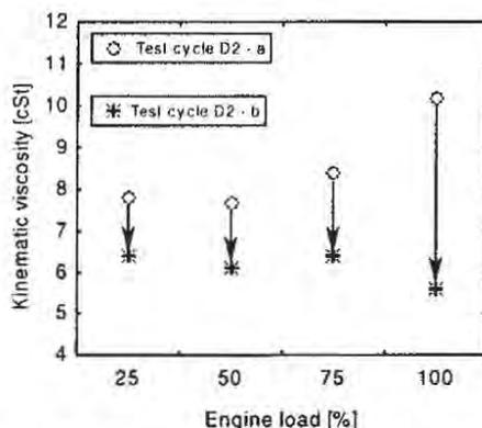
Figure 2. Fuel oil kinematics viscosity history during engine tests
